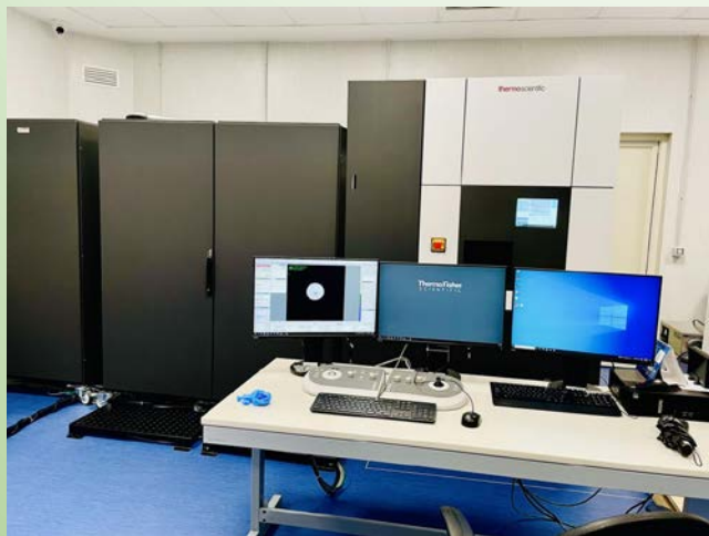
Thermo Scientific Glacios TEM 200kV (camera/detector Falcon 4i, filtro Selectris X)
